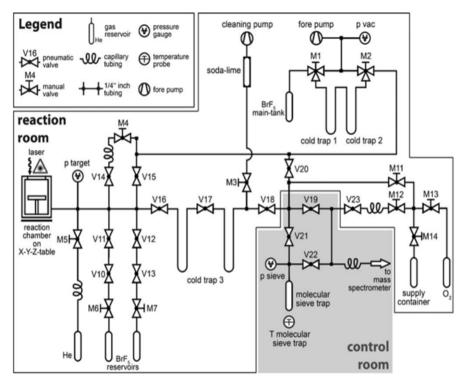
Figure 2: Valve chart of the instrumentation, set up in two different rooms
