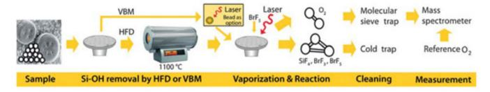
Figure 1: The removal of exchangeable oxygen - two methods were tested (Helium Flow Dehydration = HFD; Vacuum Bead Melting = VBM)
