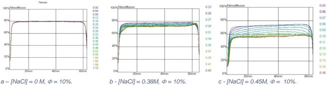
Figure 2. Effect of salt concentration on emulsion flocculation
