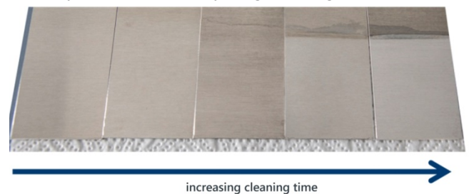
Fig. 2: Photo of steel plates after cleaning with increasing cleaning duration from left to right
